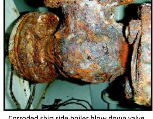
Corroded ship side boiler blow down valve
