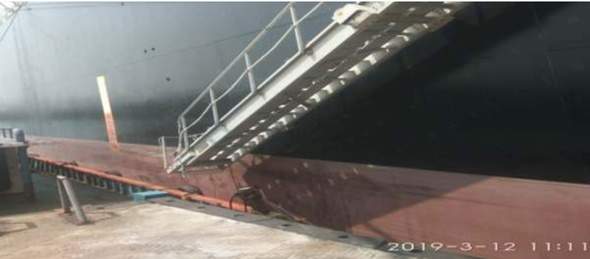
Gangway is not provided with safety net
